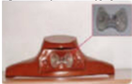
Fig. 3. The thyroid RSD type phantom
