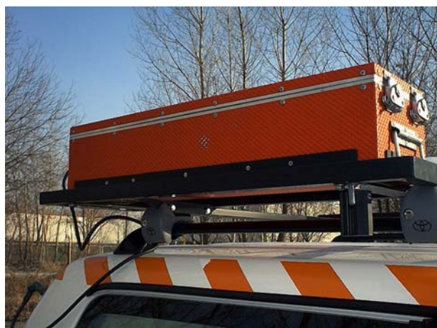
Fig. 2. GPX-256 detector with the NaI(Tl) crystal.
