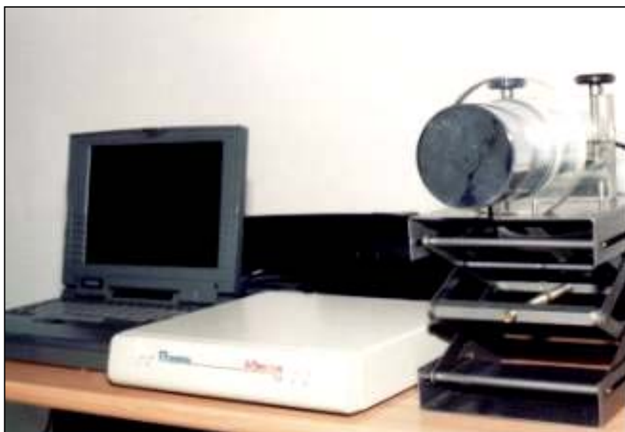
Fig.1. Mobile detection unit for I-131 measurements
