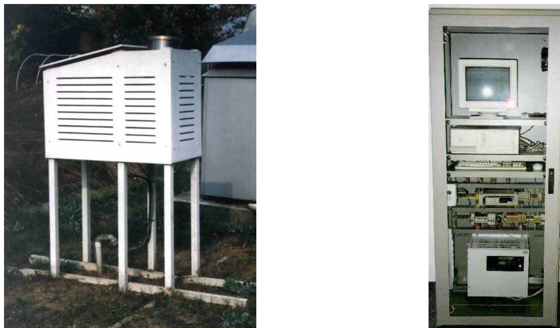
Fig. 4. PMS station (sensors and electronic parts).
