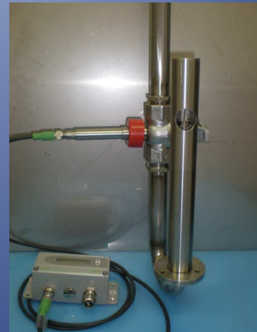
Air flow meter and air heating.
